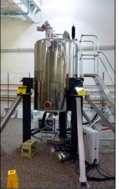
The 800 MHz NMR spectrometer is located in the D.M. Grant NMR Center, also known as the Gauss Haus.
