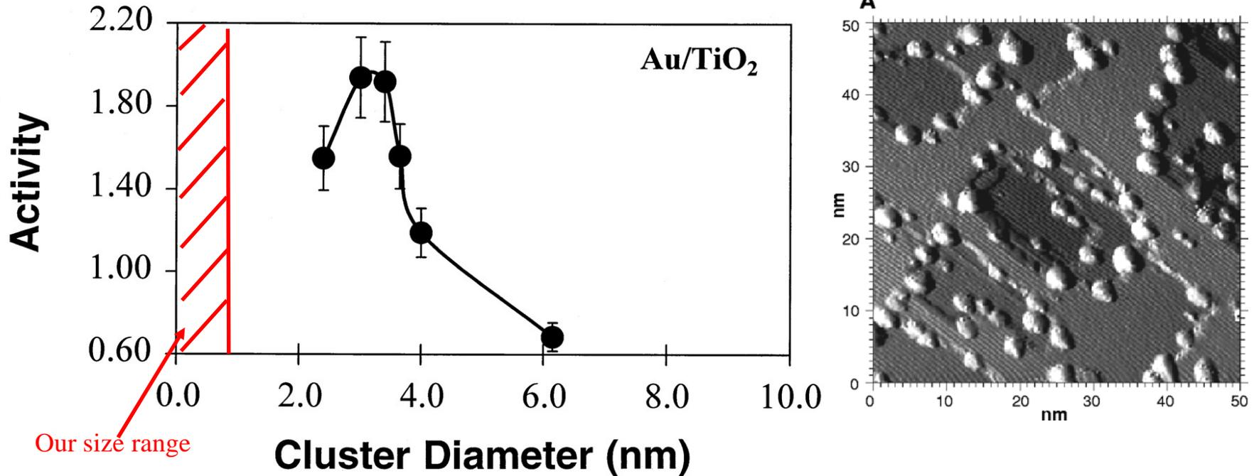
Planar model support / Cluster grown by annealing Au/TiO<sub>2</sub>
